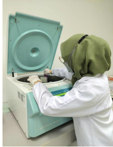
Gambar 8. Proses centrifuge sampel responden
