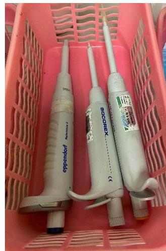
**Gambar 2. Alat mikropipet**
