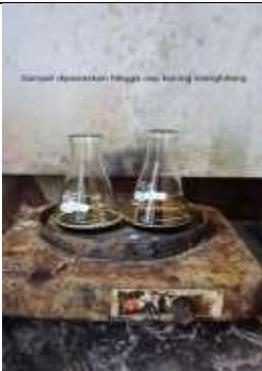
Two Erlenmeyer flasks containing a yellowish liquid are placed on a hotplate. The hotplate is a rectangular device with a circular heating area.                            | Sampel dipanaskan diatas <i>hotplate</i> hingga uap kuning menghilang. |
